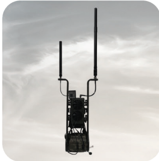
RF Jammer Module Omni-Directional Antenna System Battery
