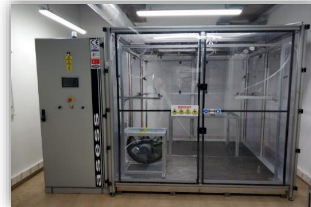
SEALING & RAIN TESTING
